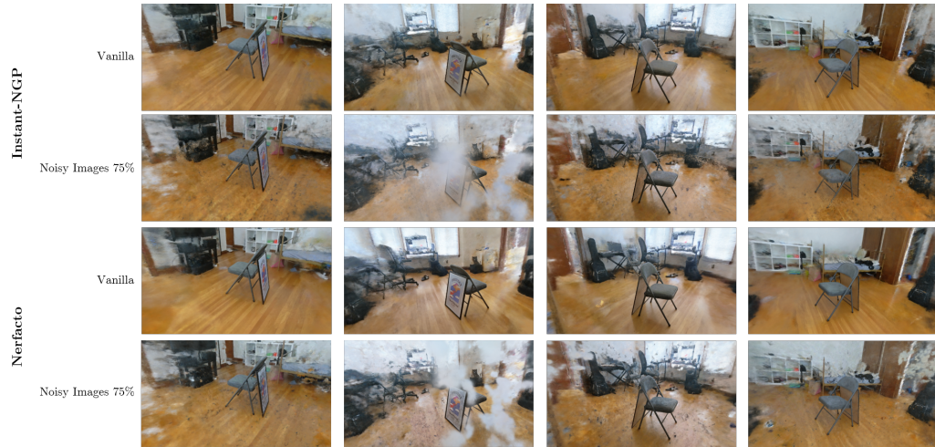
Figure 4: Some qualitative results for the indoor scene highlight the effects of compromising the image quality with coarse pepper noise.
